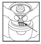
Close the mouthpiece, pull away horizontally the embossed protruding end of the strip so as to be detached, and discard it.
